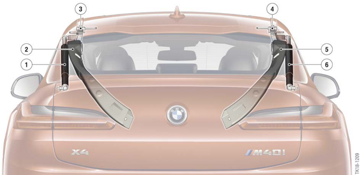
G02 tailgate with spindle drive on both sides
