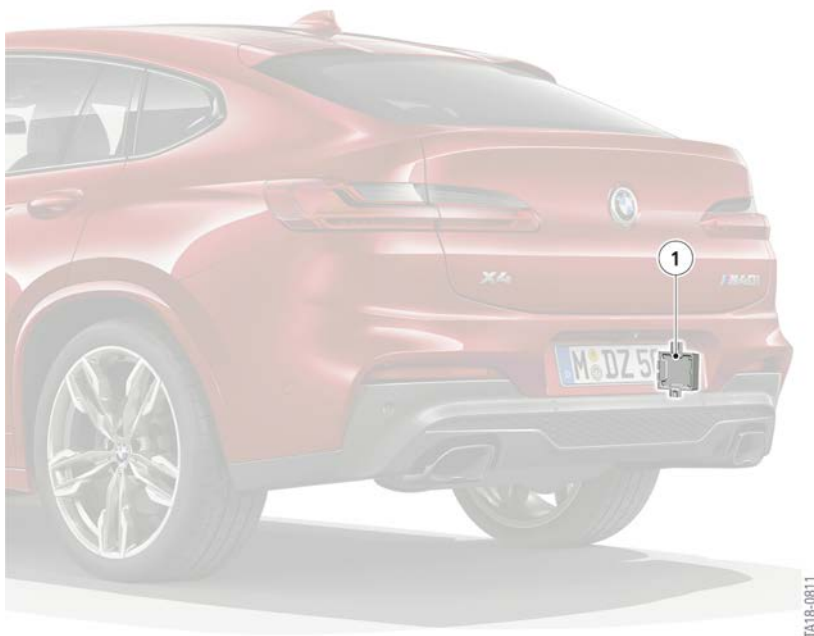
G02 mounting orientation of GHAS
